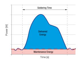
Soldering Assistant allows analyzing manual soldering processes and obtaining a qualification of these by comparing the solder joints one by one.
