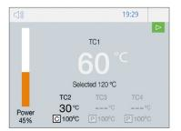
**Profile Mode** allows control of the heating rate of the PCBA by the use of a control and a protection thermocouple.
