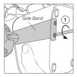
Loosen the screws (1) at the bottom.
