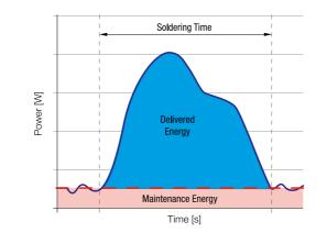
Soldering Assistant allows analyzing manual soldering processes and obtaining a qualification of these by comparing the solder joints one by one.
