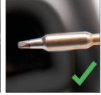
A clean tip is always easier to tin, resulting in **higher** quality solder joints.
