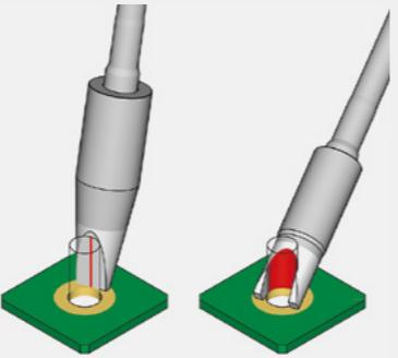
The bigger the contact surface that the tip has with the application, the higher the **thermal transfer**.
