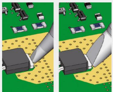
The more mass the tip has, the more heat is accumulated and the **lower is the temperature drop**.
