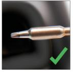
A clean tip is always easier to tin, resulting in **higher** quality solder joints.
